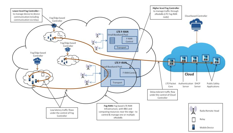
Highly Available and Resilient Network Architecture for Rapidly Deployable Public Safety Communication system
